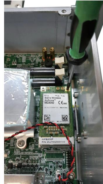
2-2. Secure the module with screws.
