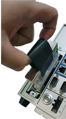
4. Install the 2.5" HDD into the bracket and secure it with screws.
