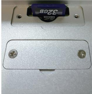
4. Ensure the SD card is correctly secured in position.
