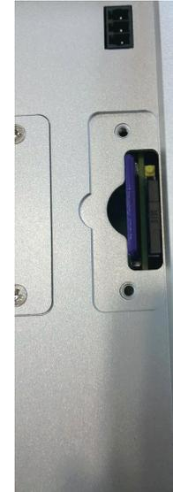
5. Press down the SD card until it is fixed into the socket.
