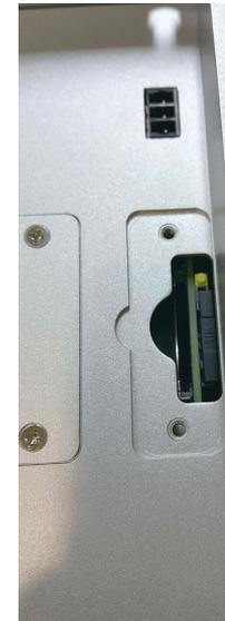
3. Insert the SD card into the SD card socket.
