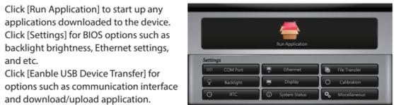
Click [Run Application] to start up any applications downloaded to the device. Click [Settings] for BIOS options such as backlight brightness, Ethernet settings, and etc. Click [Enable USB Device Transfer] for options such as communication interface and download/upload application.
